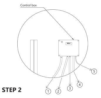
Open the control box by unscrewing the four screws on the box cover. Mount the box on the wall close enough to the rail guide so all the cables and hosing could reach the slider on the rail guide using the provided screws. Finally put the cover on and screw it.
